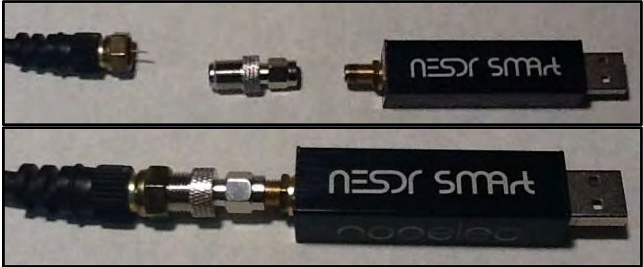
Figure 26 Connecting the antenna to the dongle. The picture above shows components before connection. The picture on the right shows three elements connected.
