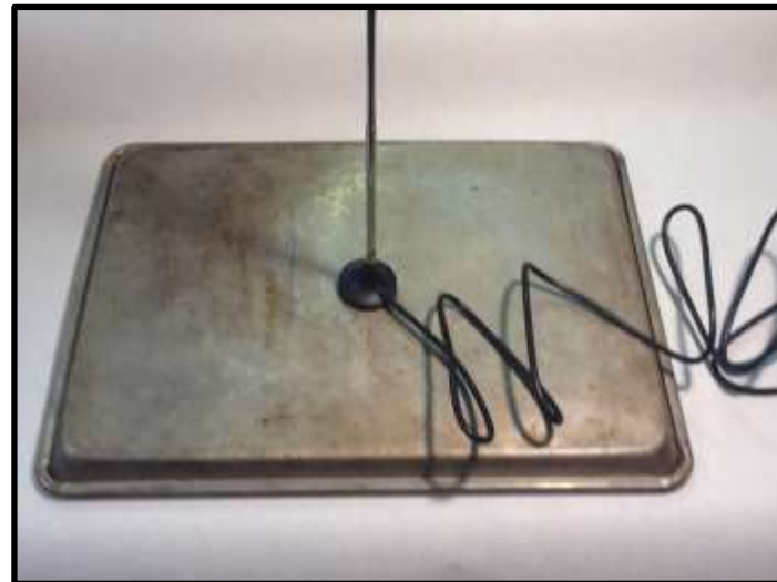
Figure 12 An example of a ground plate made from a cookie sheet.
