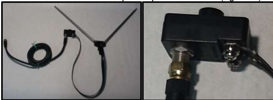
Figure 25 On the left is the complete rabbit ear set up. On the right is a close up of the connection.
