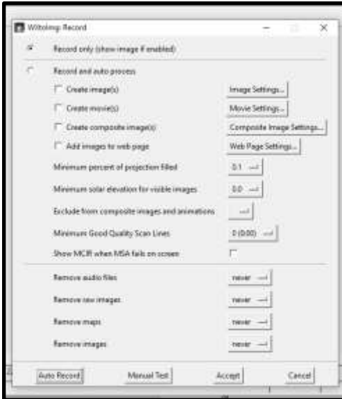
Figure 33 The Wxtolmg record window. Select the radio button. Click Auto Record.
