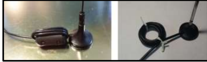
Figure 13 Examples of a simple coax choke. The image on the left uses a ferrite core while the one on the right is a simple coil.
