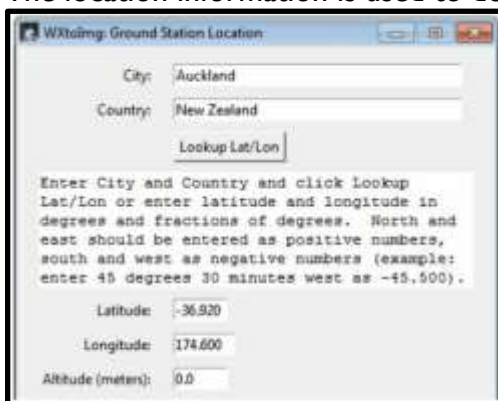
Figure 31 Setting up the location of the ground station.
