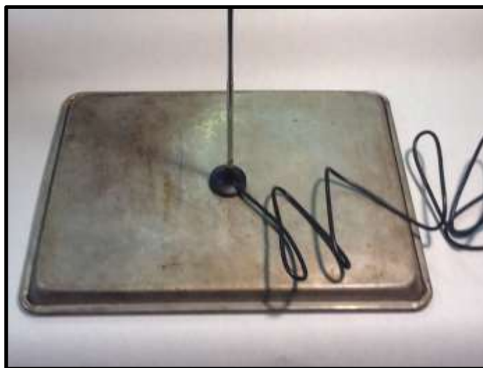
Figure 12 An example of a ground plate made from a cookie sheet.
