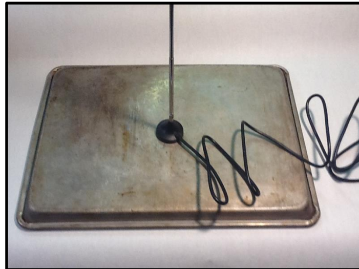
Figure 12 An example of a ground plane made from a cookie sheet.
