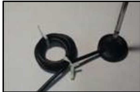
Figure 13: A simple coax choke made from a circle of cable.
