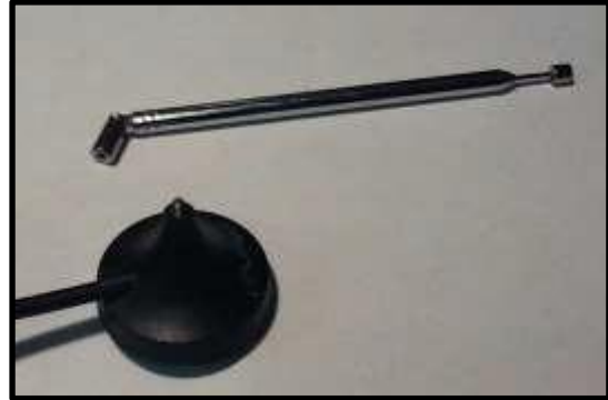
Figure 1 The telescoping antenna (above) and threaded base (below)
